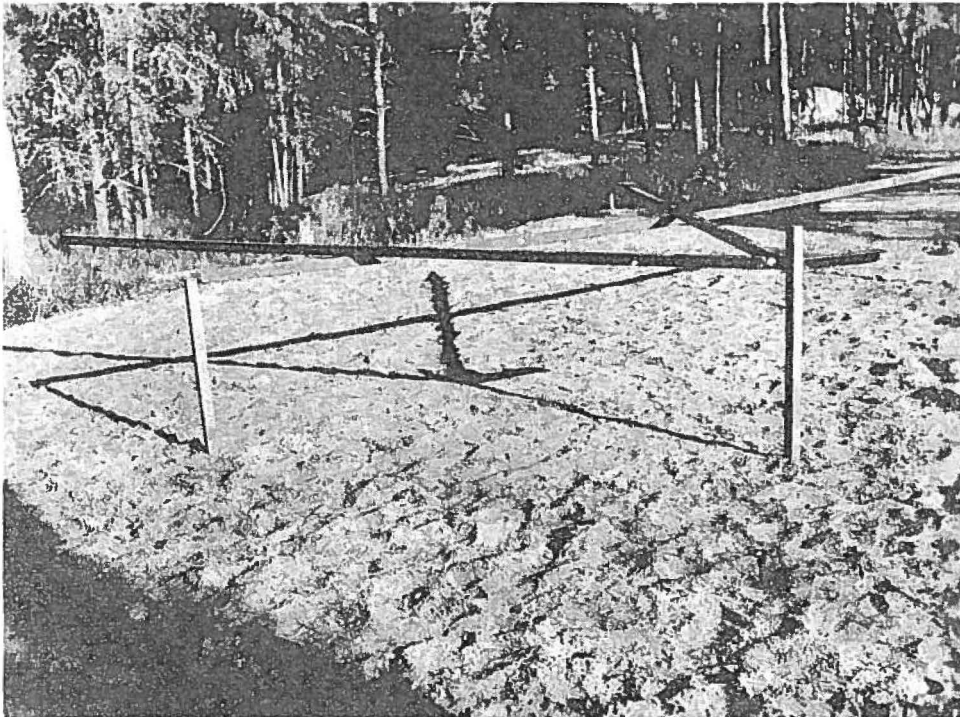
Fig. 6 Jig used for locating positions of moss-filled traps in the field.
