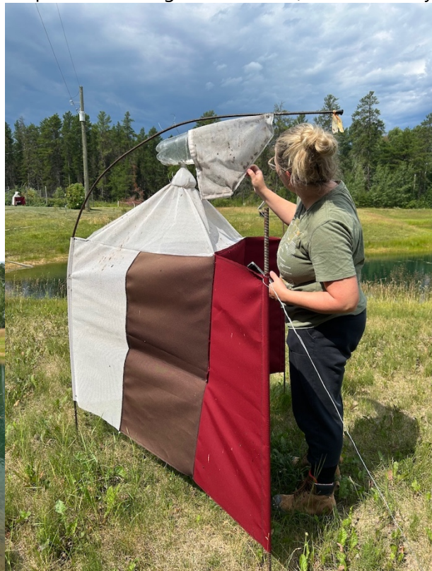
Lisa examining the Bossenmaier fly trap, which efficiently captures great numbers of biting flies.
