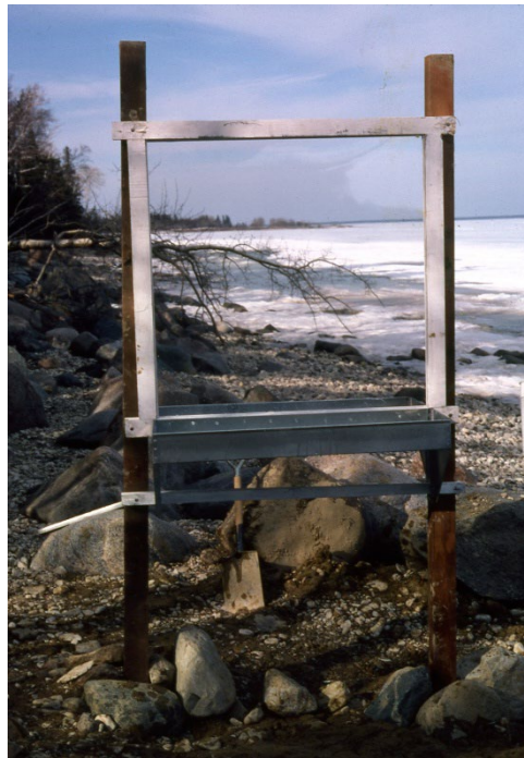
Figure 1. Window trap installed on a beach on Hecla Island, Manitoba.
